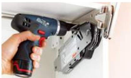
The lift force can be adjusted (according to the frontal weight) using a power screw driver (Pozidriv®, size 2, length 39 mm). To make adjustment easier all AVENTOS mechanisms include a calibrated scale.
